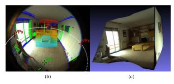
Fig. 1: (a) Fields of view of our proposed system composed by a Fisheye and a RGB-D camera. (b) The depth information in the center is extended to the periphery combining information with the line segments that we use to extract the spatial layout of the scene. (c) At the end we obtain a 3D reconstruction of the scene with scale.
