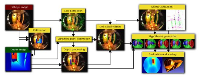
Fig. 2: Block diagram of the main stages of the algorithm, starting with the initial Fisheye and Depth images and finishing with the result of the evaluation.
